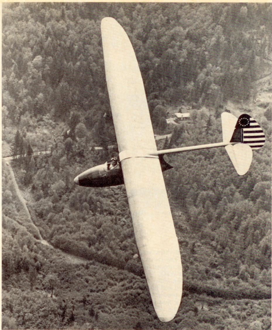
Bowers in his Bowlus Baby. Note the "horseshollar" canopy, which is put on after the pilot is seated. Photo by Jim Larsen.
